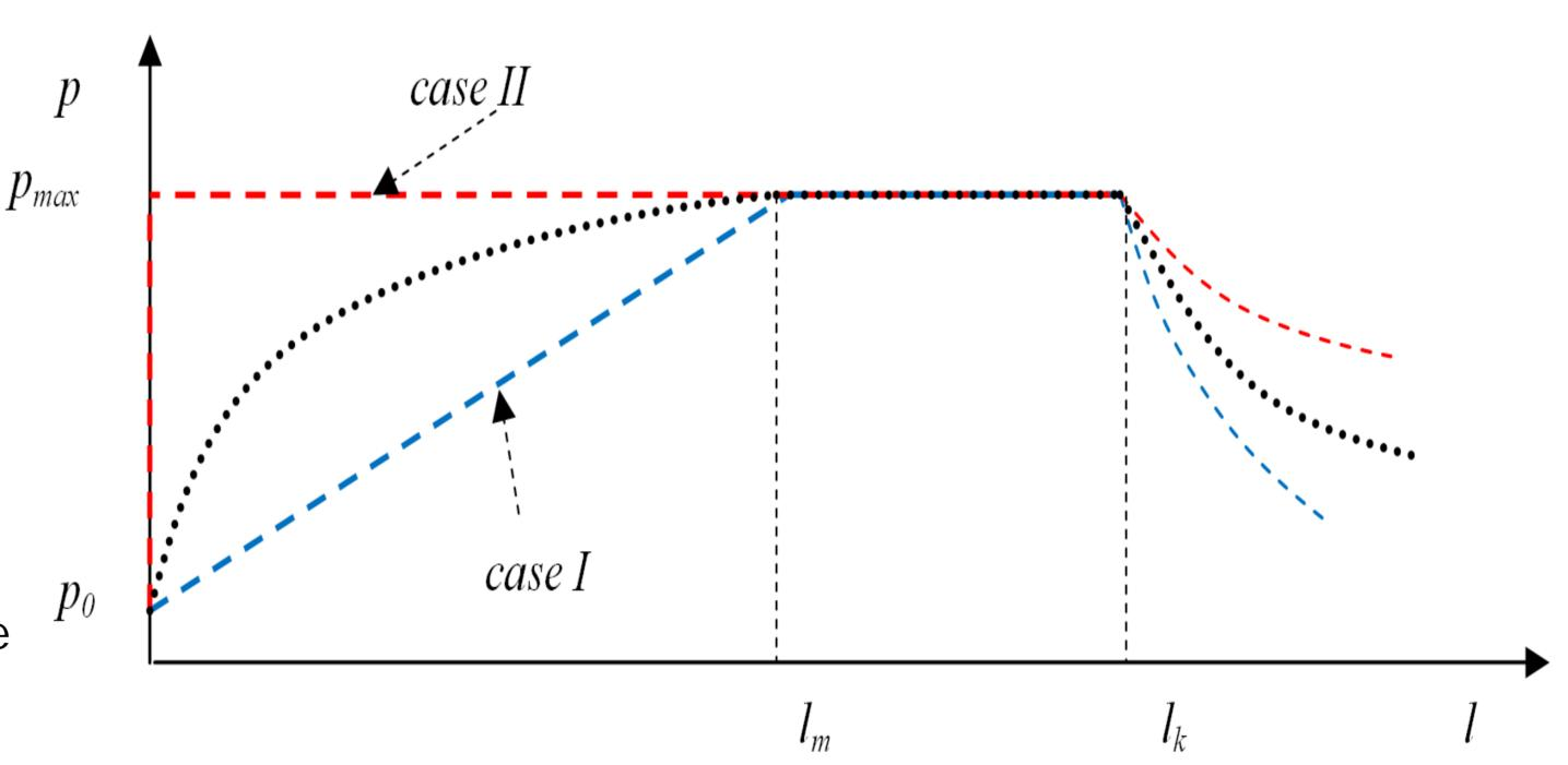
For the analysed gun system, there is not possible to reach a constant pressure plateau when is used a propellant characterised by a single set of geometrical characteristics over the entire web thickness
