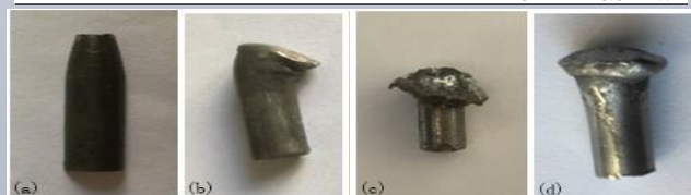
Recovered cores from ballistic tests, (a) original core; (b) recovered from C3+12; (c) recovered from C5+10; (d) recovered from C0+20
