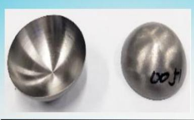
Tantalum zirconium liner is a kind of dual phase liner which is mainly composed of tantalum and zirconium. The shaped charge warhead equipped with such charge liner can effectively break through the amar, and cause extra ignite/detonate effect via combustion of the Zr element.
