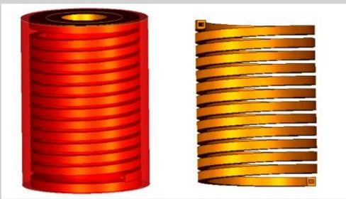
Fig. 2 Structure of the Solenoid Pulsed Inductor
