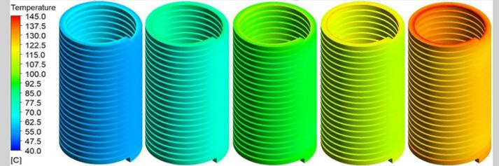
Fig. 4 shows the temperature distribution at the end of the 1st, 4th, 6th, 8th and 10th discharge of solid coil inductor. The temperature of solid coil inductor increases with the increase of discharge times. The peak temperature is close to 145 °C, which exceeds allowable peak temperature of pulse inductor, indicating that the natural cooling conditions cannot meet the temperature control requirements of continuous discharge of designed PFU.
