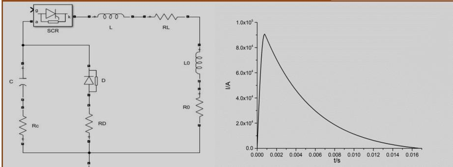
Fig. 1 Circuit Model and Discharge Current Curve of 250kJ PFU
