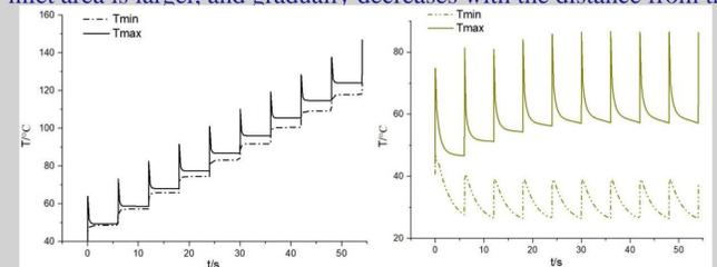
Fig. 6 Curves of Maximum and Minimum Temperature of Solid Coil Inductor (Left) and Hollow Coil Inductor (Right) during Continuous Discharge
