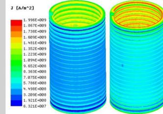
Fig. 3 Current Density Distribution of Solid Coil Inductor (Left) and Hollow Coil Inductor (Right)
