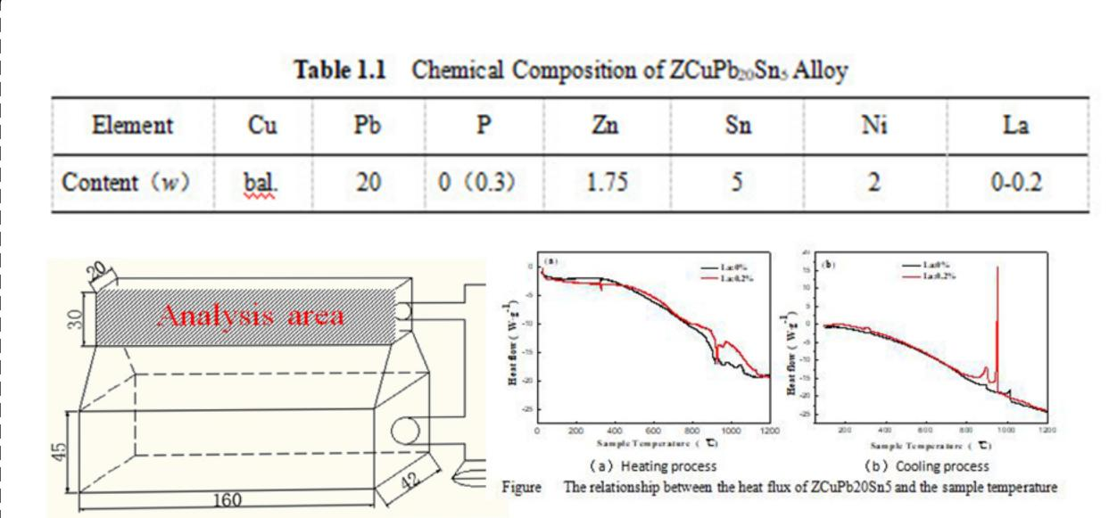
The casting temperature of ZCuPb20Sn5 alloy is 1200±20°C, and the casting test block is a copper alloy metal mold casting test block. Please refer to the national standard GB/T 1176-2013. The etching solution is continuous hydrogen peroxide, ammonia and water in a ratio of 1:1:1.
