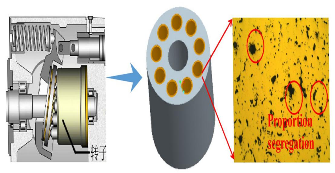
Due to the difference in density between lead and copper, the specific gravity segregation of lead is easy to occur during solidification, which leads to the instability of alloy properties.
