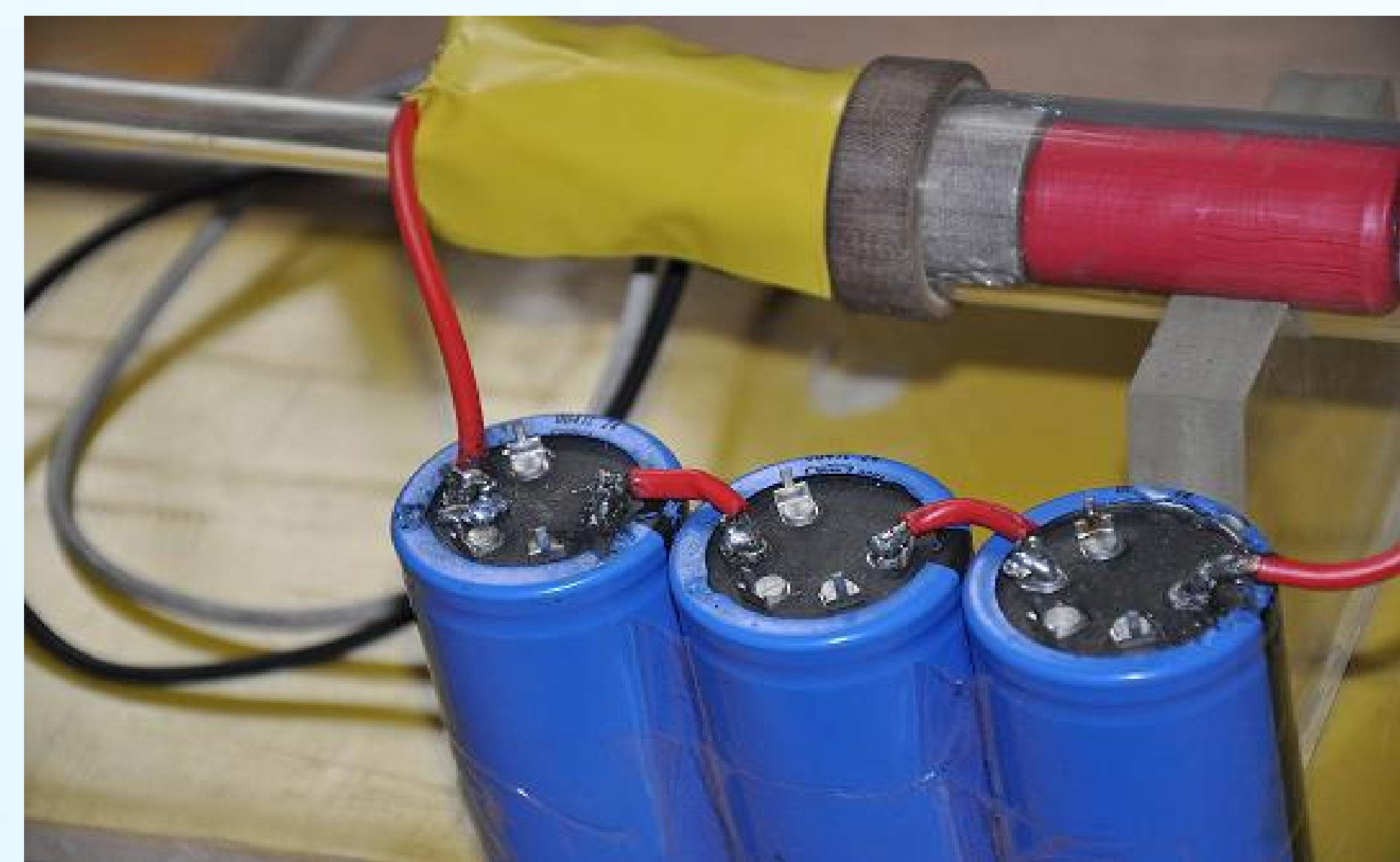
Test device diagram of a single-stage reluctance coil launcher
