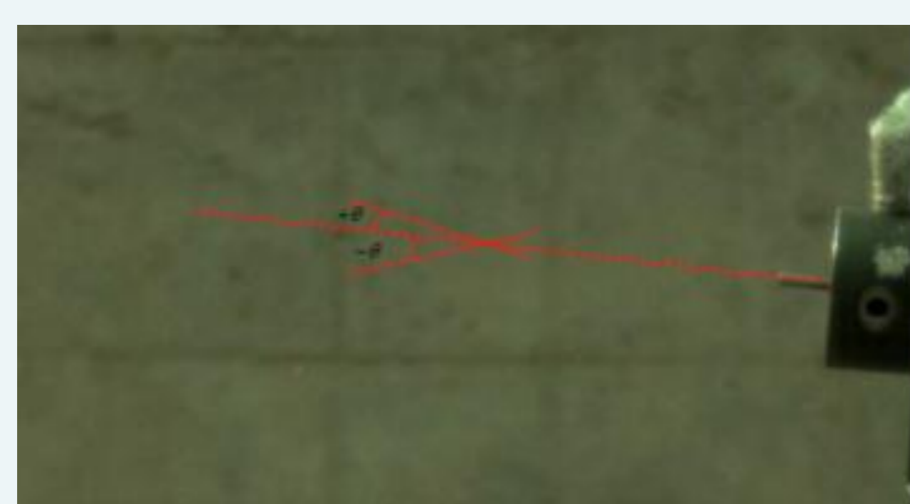
•Fig. 3 Schematic diagram of the projectile pitch inclination
