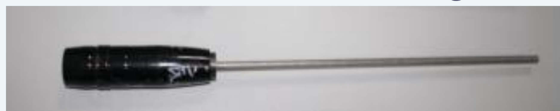
•Fig. 1 Projectile for testing the initial ballistic characteristics of the CTA
